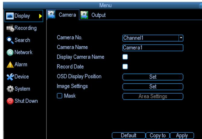
**Camera No.:** Choose the camera / channel you want to edit here. The Camera No is the same thing as the number written on the rear panel next to the BNC socket used to connect the camera.
