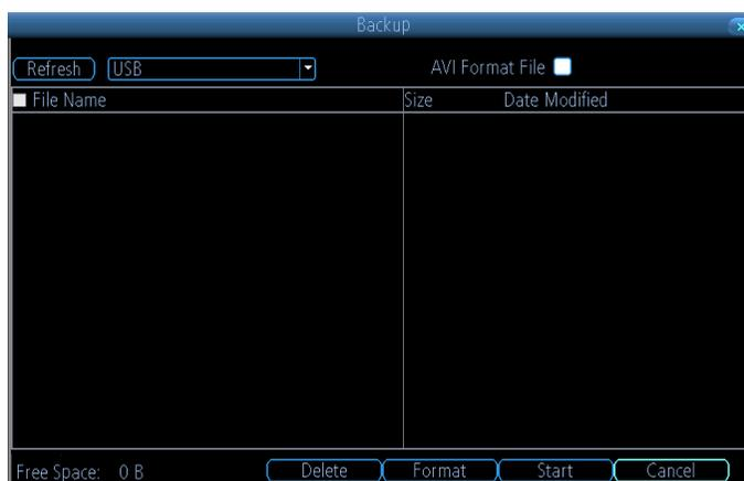
**Refresh:** Looks for devices to which footage can be backed up. This will include USB flash drives or hard drives connected to the USB port, or external hard drives connected via the rear eSATA port.
