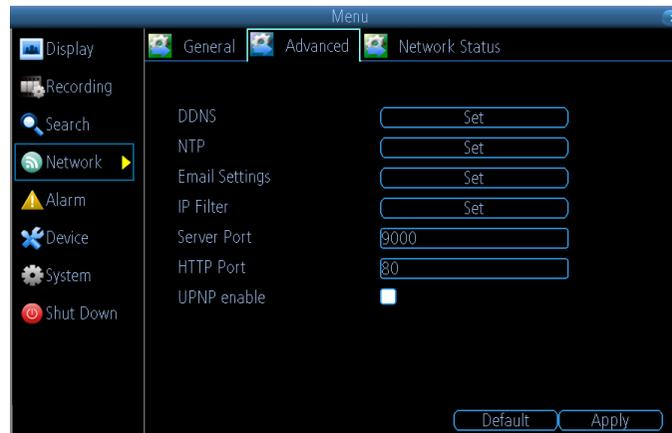
**DDNS:** The place to configure the DVR to automatically update a dynamic DNS service. If you want to remotely access the DVR via the Internet, you'll probably need to configure a DDNS account. See "Network: Advanced: DDNS" for details on setting up and configuring the DDNS.
