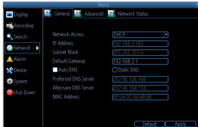
**Network Access:** Here you can choose between the three different types of networks that the DVR can be connected to. The three types of networks are:
