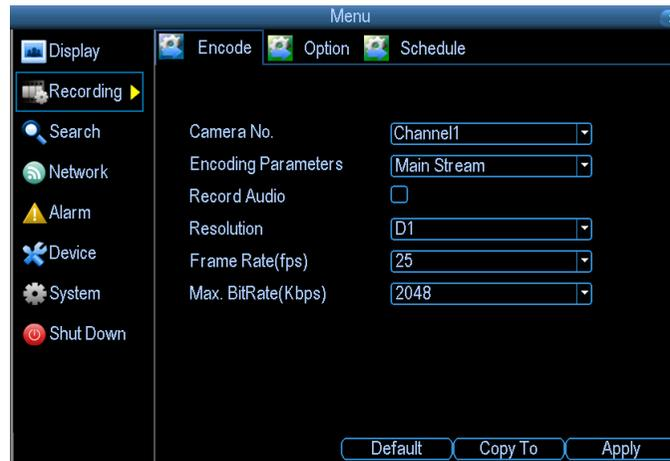
**Camera No.:** The camera feed you want to alter the settings for. These will be numbered sequentially, and correspond to the BNC video inputs labeled on the rear of the DVR. Note that the channel name here is independent of the Camera Name selected on the Display: Camera menu screen.
