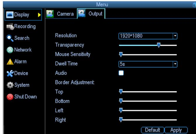
**Resolution:** Resolution should be set as high as possible, but equal to or lower than the maximum resolution your screen/monitor can display. Things change a little depending on what kind of monitor you're using, and how it's connected.
