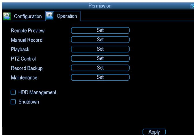
Choose the Set button next to each type of access to choose specific channels that the user can access. Also, this page contains permissions for HDD Management and Shutdown. These are surprisingly powerful levels of access: between them, a user can remove all footage from a DVR's hard drive and turn the DVR off. Be careful assigning these permissions!
